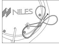
Figure 10 Security Cable after Looping
